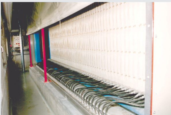
filter press for cake drying with membrane chamber plates 1200 x 1200 mm
